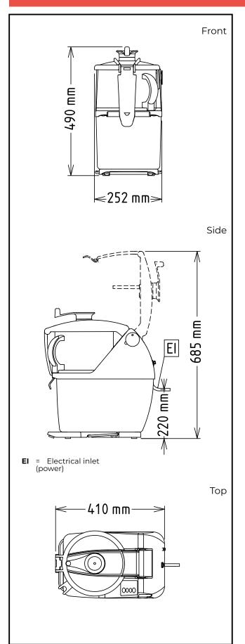
Electric Supply voltage: 200-240 V/1N ph/50/60 Hz Electrical power, max: 1 kW **Total Watts:** 1 kW Capacity: Performance (up to): 550 kg/hour **Capacity:** 4.5 litres Key Information: External dimensions, Width: 252 mm External dimensions, 485 mm Depth: External dimensions, Height: 505 mm **Shipping weight:** 30 kg
